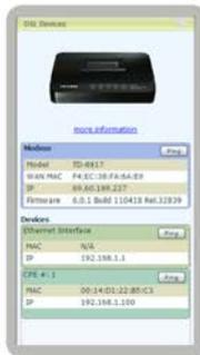
**DSL Device Panel.** Displays the modem MAC address. If TR-069 enabled see the model #, IP, firmware level, plus IP/MAC for interfaces/devices
