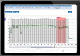
SpectraVizion provides a proactive view to your downstream spectrum analysis, giving your staff the ability to see which subscribers are being impacted by downstream issues in your cable plant
