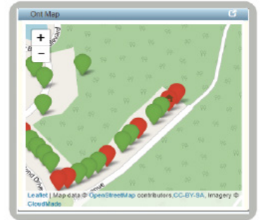
Intelligent Mapping Map panel shows locations of ONTs color coded by issue severity
