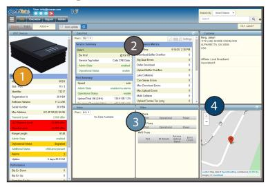
See optical levels, errors (BIP, GEM, Burst) and easily see any alarms for the ONT, color coded by alert level. Click to graph this data over time.
